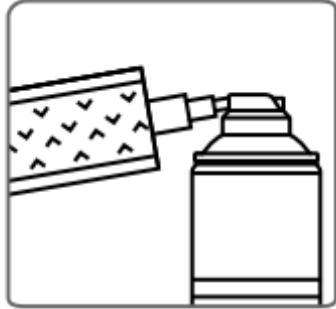
Lubricate the handpiece after each cleaning and before each sterilization cycle. Henry Schein® recommends using Henry Schein® Spray & Clean (102-8721), KaVo Spray or an equivalent lubricant spray.
